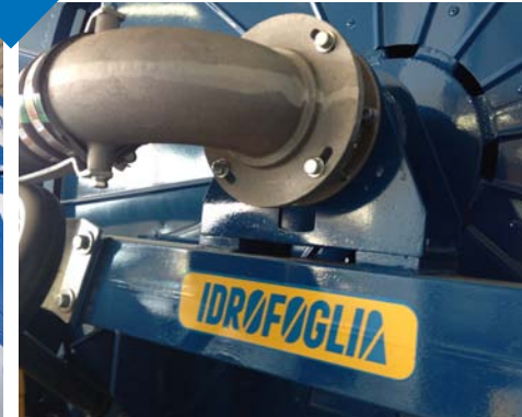
Inlet water joint.
