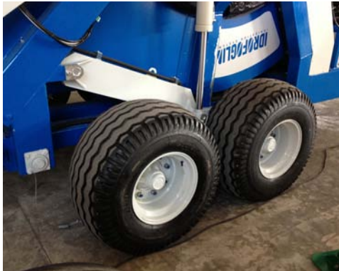
Twin-axle for 4 wheels frame mounted under drum centre of the hose reel for easy moving.
