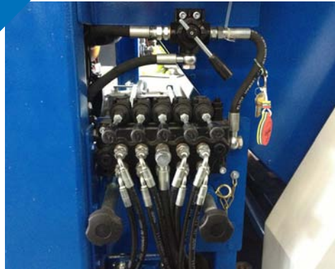
Hydraulic distributor levers to move and position the machines.
