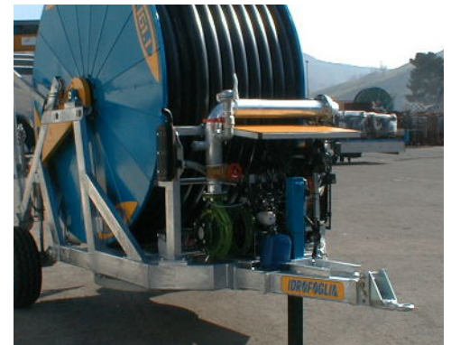
Motor pump for pressure boost.
