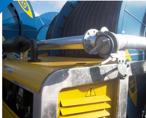
Secondary water inlet.
